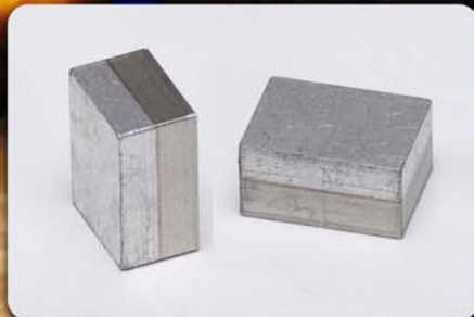
Explosively welded aluminum to stainless steel
