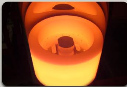
Vacuum Brazing copper to stainless steel
