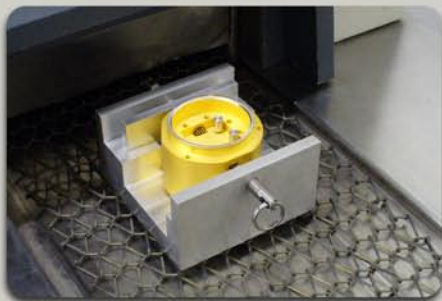
Conveyor Furnace Brazing in a hydrogen atmosphere
