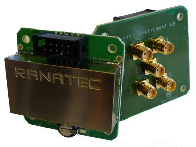
Ranatec RI 2441 is a high performance SP4T solid state switch module suitable for high volume switching applications.
