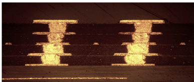
Scan shows 4 stacks of microvias and the adjoining finely etched traces.
