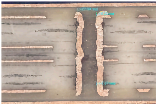
fastRise bonding a top and bottom cap dielectric layer and simultaneously via filling 13K buried vias, 28 mil deep.
